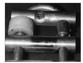
Rack spacer and worn hollow brake bar
