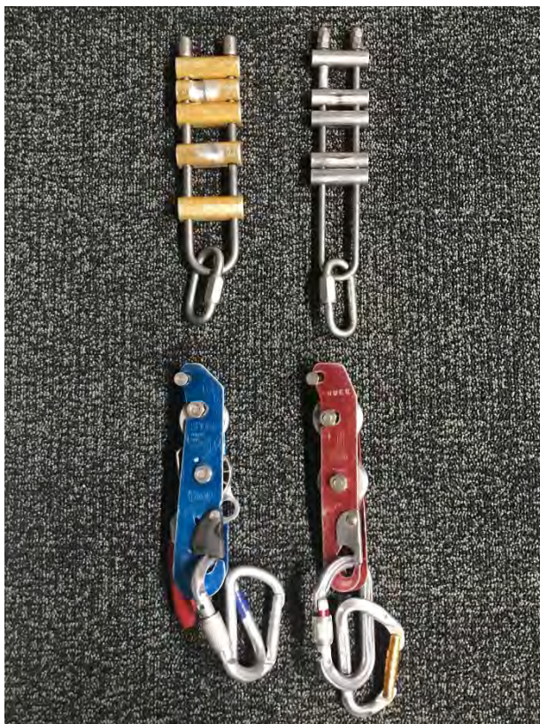
Descender options in the storeroom (L-R, T-B): SRTE 5-bar aluminium rack, Aspiring 5-bar stainless steel rack, Petzl Stop, Petzl Simple (photo by Lachie Bailey)
